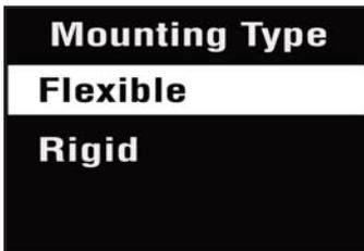
As a basic "rule of thumb", unless a machine is bolted down to a concrete floor, its mounting should be considered as being **flexible**.
