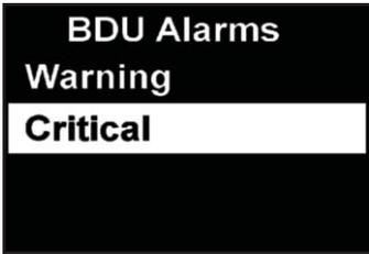
The BDU threshold values are designated as Warning (where readings turn **Amber**) and Critical (where readings turn **Red**).
