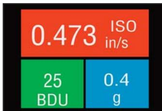
Taking a reading causes the overall vibration numbers screen to be displayed as shown in the example screen left.
